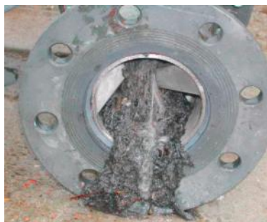
Typical clogging of competitor's mixer after less than 5 hours
